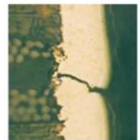
Crack 裂缝(内层/电镀层)
