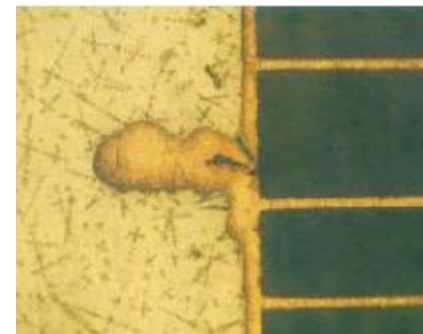
Plating Nodule 孔内铜瘤
