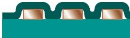
Soda Straw 吸管空隙
