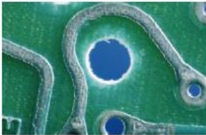
Soda Straw 吸管空隙
